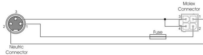
For both Off-board and On-board Charging, the maximum charging current is 9A rms. Refer to Section 3 of this chapter for pin-out details of this connector.
