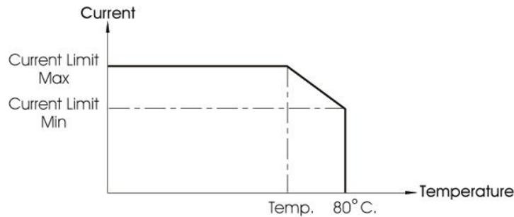
If the S-Drive's internal temperature reaches the value set by Current Foldback Temp., then the maximum current output will be reduced from the value set by Current Limit Max. The reduction will be a linear reduction to a value set by Current Limit Min. at a fixed internal temperature of 80°C.
